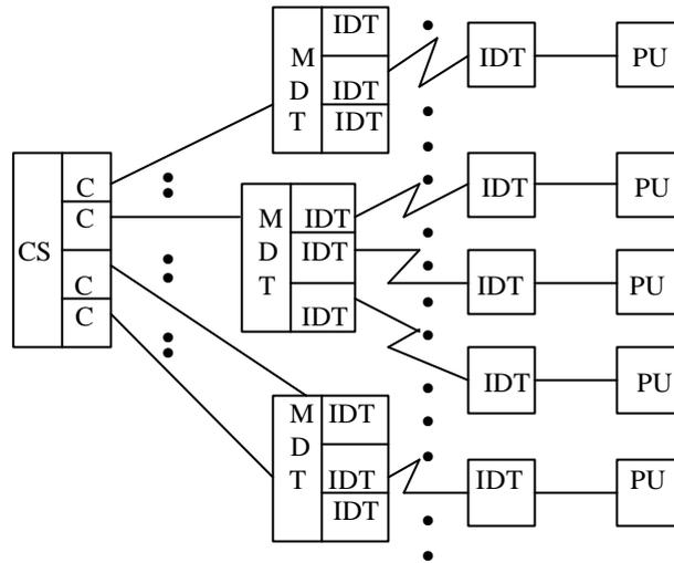
Fig. 1.6. A system of data teleprocessing.
