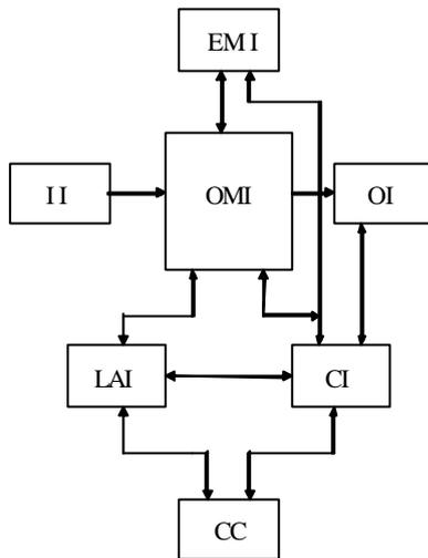
Fig. 1.1. Logical structure of a first-generation computer.
