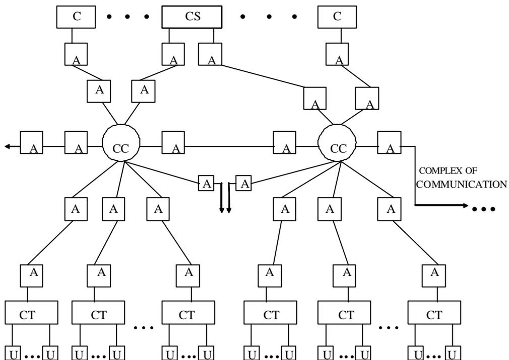
Fig. 1.7. Structure of a computer network.
