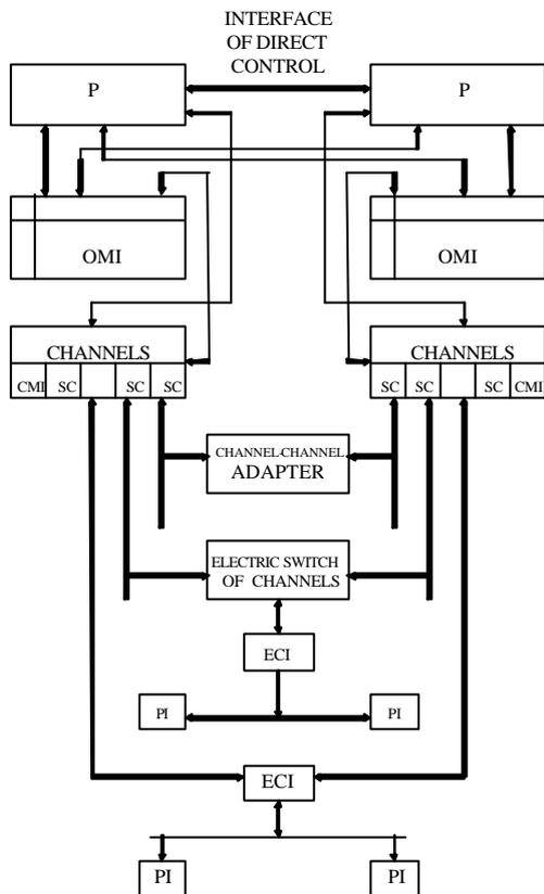
Fig. 1.3. Levels of interconnection of two computers joined in a single computational system.
