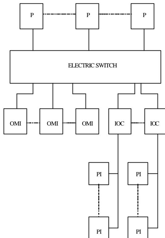
Fig. 1.4. Computer system of multiprocessing.
