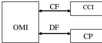
Fig. 1.10. Organization of a CS of multiprocessing, according to the principle UCUD. CCI - central control of installations; CP - central processor; CF- command flows; DT - data flows.
