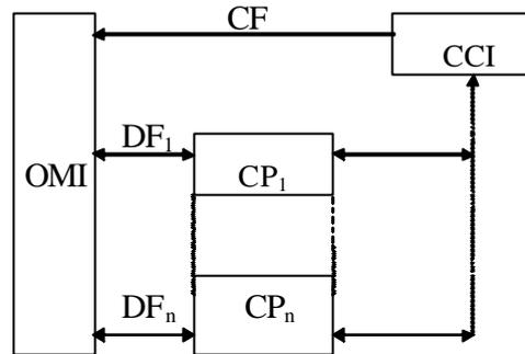
Fig. 1.11. Organization of a CS of multiprocessing, according to the principle UCSD.
